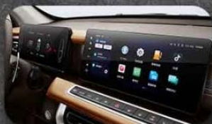
7 inch LCD instrument panel + 12.3 inch smart central control
